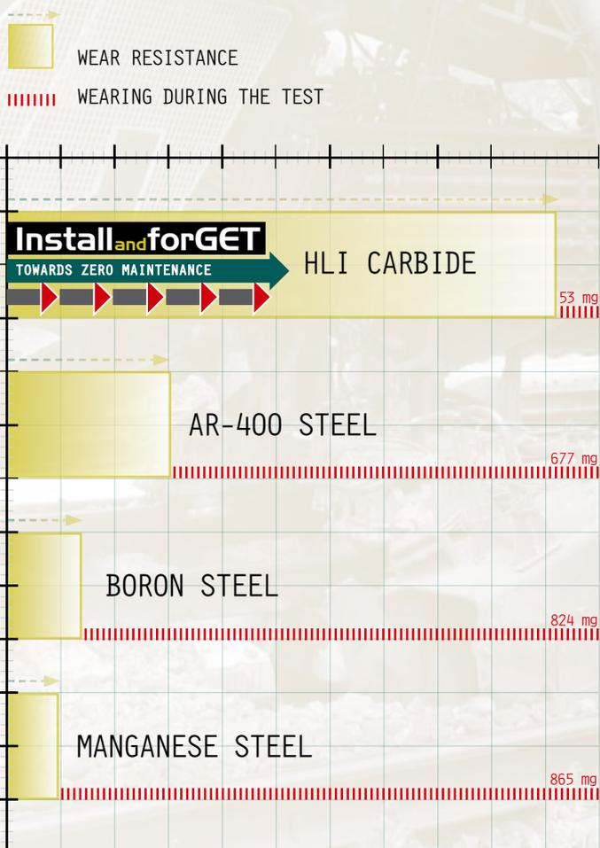
RUBBER WHEEL ABRASION TEST CARRIED OUT ACCORDING THE STANDARD ASTM G-65.
